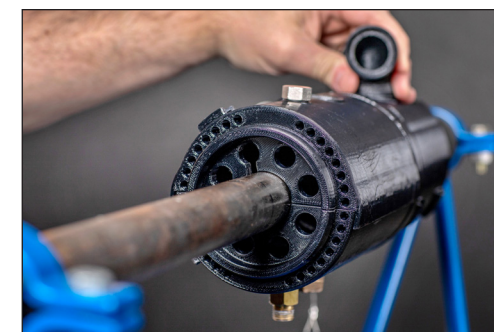
Vortex freeze sleeve. (PSNS & IMF photo by Scott Hansen)
