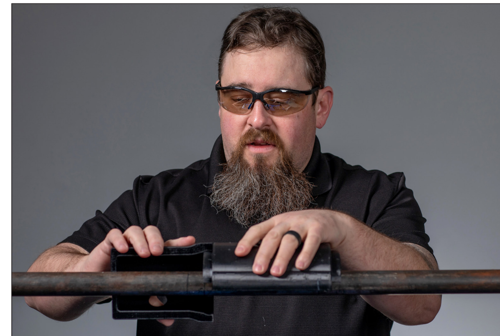
Mitch Van Epps with Code 1010, Reactor Systems Product Line sets up the 3D printed vortex freeze sleeve display model. (PSNS & IMF photo by Scott Hansen)
