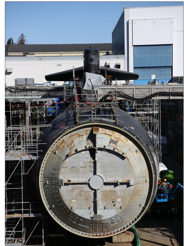
Ex-Buffalo (SSN 715) sits in Dry Dock 1 at Puget Sound Naval Shipyard & Intermediate Maintenance Facility in Bremerton, Wash., with the sonar dome and sonar transducers removed, March 5. (PSNS & IMF photo by Max Maxfield)
