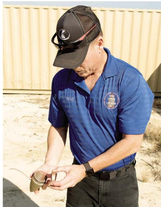
Wolf Amacker, Fort Bragg installation range officer, inspects the nose cone of a 2.75 inch rocket that was fired on the new aerial gunnery range. The rocket contained approximately 2,200 20 grain flechettes. Flechettes are small steel darts that disperse in front of a target and then penetrate vehicles and light armor.
