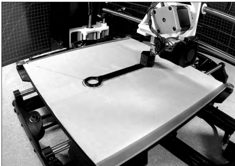
This photo shows a 3D printer producing six-inch cap, used to protect the fire extinguishing system housed the wheel wells of Mine-Resistant Ambush Protected vehicles. Soldiers in Korea identified a fire-suppression cap degradation issue and turned to 3D printing technology for help. The team requested engineering support from the Armament Research, Development and Engineering Center at Picatinny Arsenal, New Jersey. (Photo by U.S. Army)
