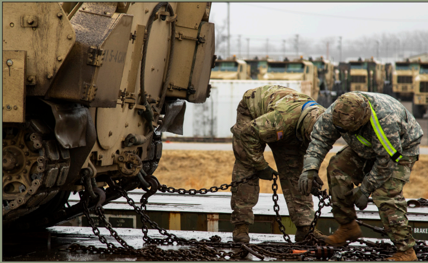
Sgt. Jimmy Tibiri and Sgt. Nicholas Harper, both with 2nd Armored Brigade Combat Team, 1st Infantry Division, attach links securing their Bradley Fighting Vehicle to a flatcar, Feb. 11. A secure attachment to a is important for a safe trip to the National Training Center at Fort Irwin, California, where the brigade will train with their own vehicles and equipment.
