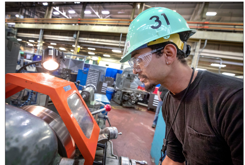
Jacob Flores, a machinist with Shop 31, the inside machine shop, uses a fixed chuck guard to protect himself while using a lathe in Building. 431, Jan. 24, at Puget Sound Naval Shipyard & Intermediate Maintenance Facility. (PSNS & IMF photo by Scott Hansen)
