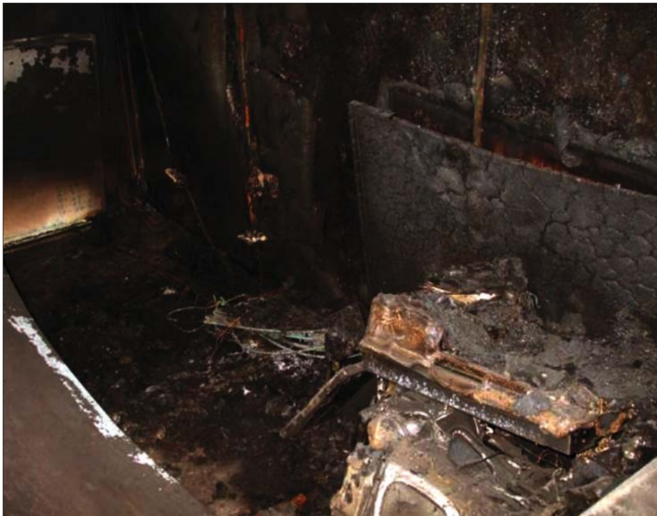
A recently burned CHU with the remains of a television in the bottom right and bed on the left after a fire caused by faulty wiring.
