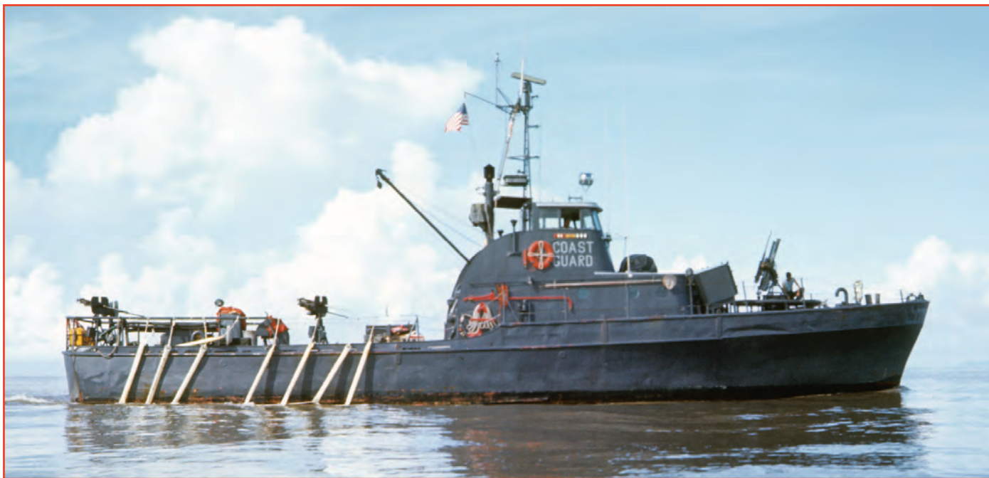
Profile view of Coast Guard Cutter Point Cypress showing 50-caliber machine guns mounted on the fantail and amidships with 81mm mortar/50-caliber combination mounted on the bow.
