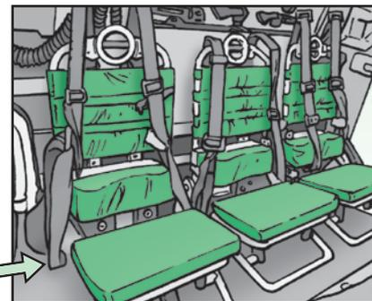
THE FOOT REST RAILS, NSN 2540-01-588-8869, CAN ALSO BE DAMAGED BY ITEMS PLACED UNDERNEATH THE TROOP SEATS.
