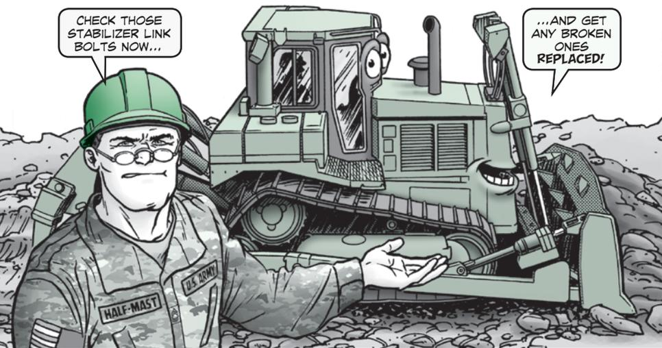
**O**perators, take a minute to eyeball the condition of the Grade 5 mounting bolts on your D7R II dozer's stabilizer link.
