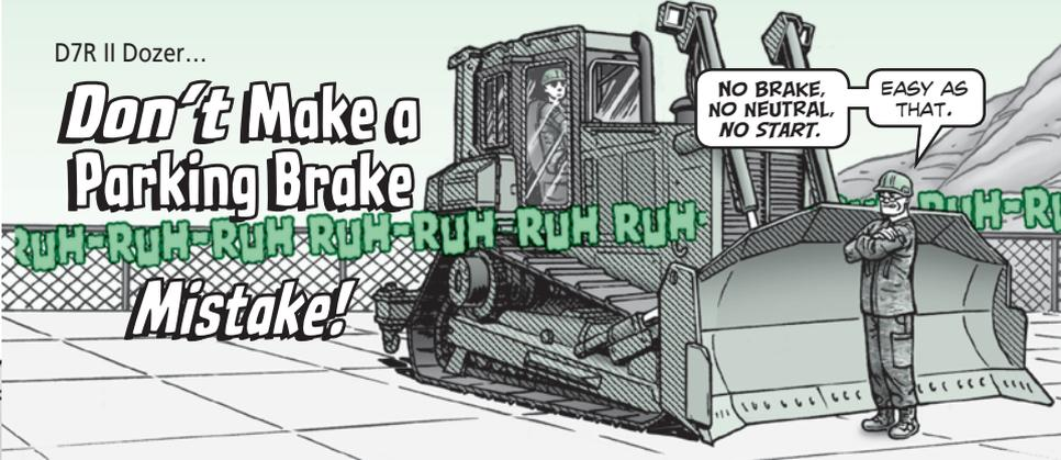
**O**perators, it's a real easy mistake to make: You hop in the cab and start cranking on the engine starter, but your D7R II dozer doesn't start and you're going nowhere.
