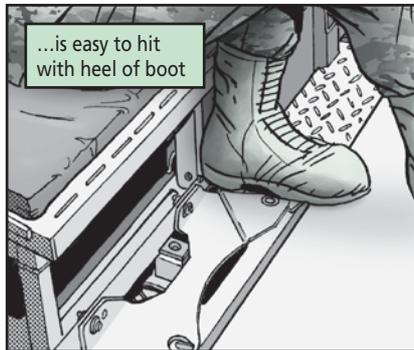
A damaged or loosened cable won't allow the vehicle's batteries to charge. So a quick check of the W4 cable might just get those batteries recharging in a hurry.
