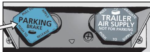
Make sure parking brake on disabled vehicle is disengaged
