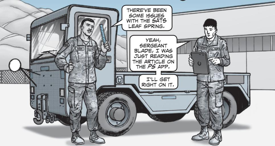
Mechanics, the leaf spring assemblies on the standard aircraft towing system (SATS), NSN 1740-01-575-5662, are experiencing excessive wear that can put the SATS in a non-mission capable status.
