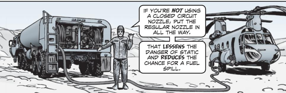
THAT LESSENS THE DANGER OF STATIC AND REDUCES THE CHANCE FOR A FUEL SPILL.
