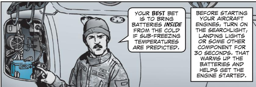
YOUR BEST BET IS TO BRING BATTERIES *INSIDE* FROM THE COLD IF SUB-FREEZING TEMPERATURES ARE PREDICTED.
