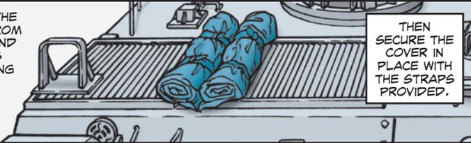
THEN SECURE THE COVER IN PLACE WITH THE STRAPS PROVIDED.
