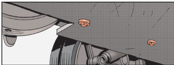
Open all three hull drain plugs to drain water (third plug not shown)
