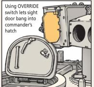
Editor's note: The OVERRIDE switch is not for normal operations. Don't use it as a shortcut or your unit could end up paying out big bucks for repairs.
