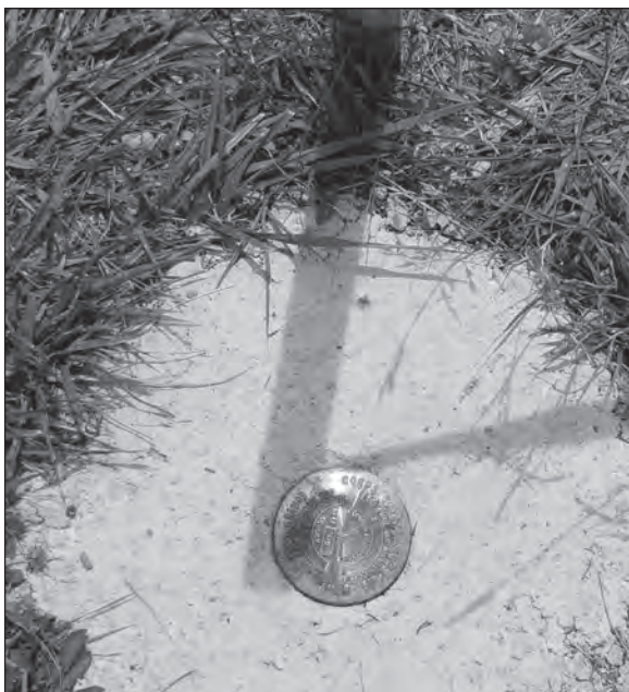
Figure 1. Standard control monument—a USACE brass survey disk mounted in concrete
