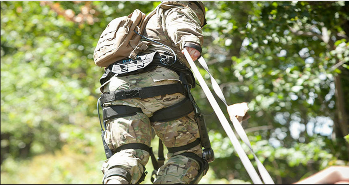
Courtesy photo The Natick Soldier Research, Development and Engineering Center is working with Lockheed Martin Space and Missile on a human augmentation system prototype. Trademarked under the name "ONYX," the system is a powered, knee-based, mobility enhancing device that shows potential for allowing Soldiers to stay in contact while maintaining peak performance longer, with equal or increased warfighting power.
