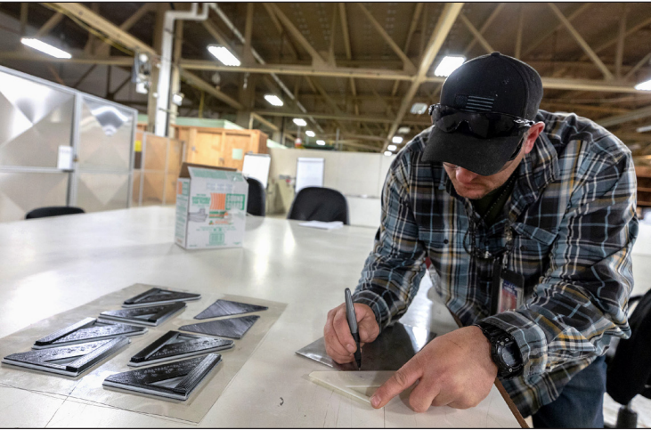
Fred McFarlane, Shop 11 shipfitter, demonstrates the use of a marking square. (PSNS & IMF photo by Scott Hansen)
