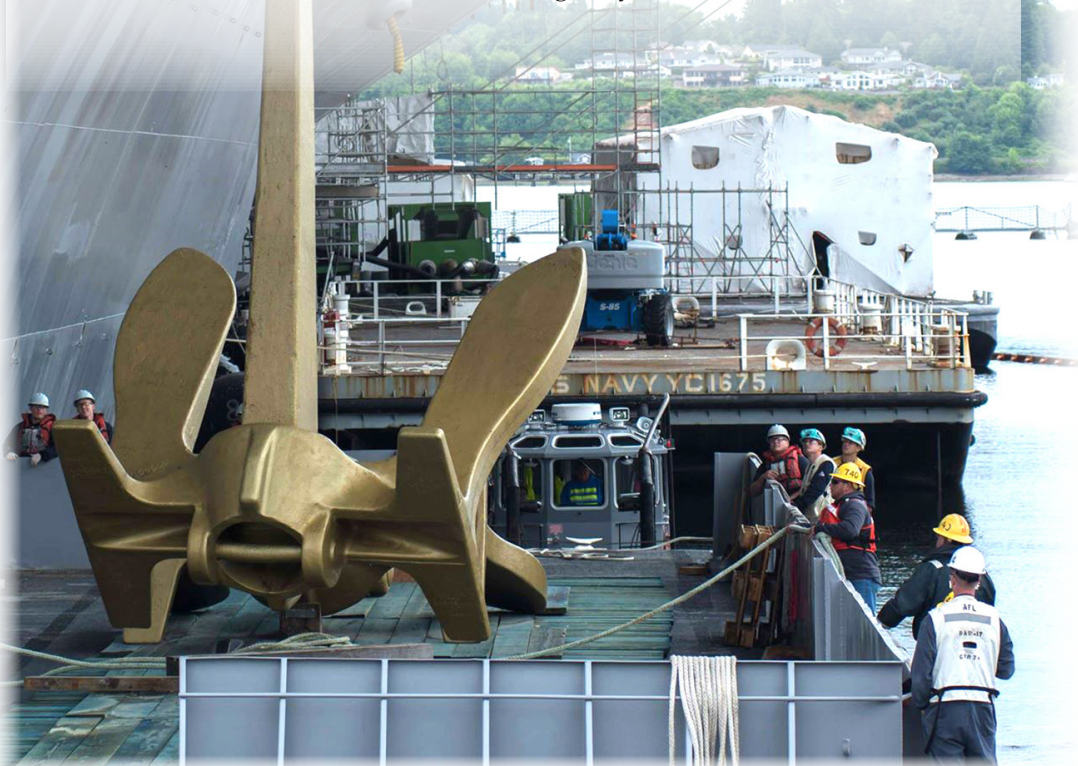
PSNS & IMF teammates and Sailors assigned to USS John C. Stennis (CVN 74) reattach an anchor to the ship's port anchor chain. The anchors were detached for maintenance and repainting. (U.S. Navy photo by Mass Communication Specialist 2nd Class Nick A. Grim)
