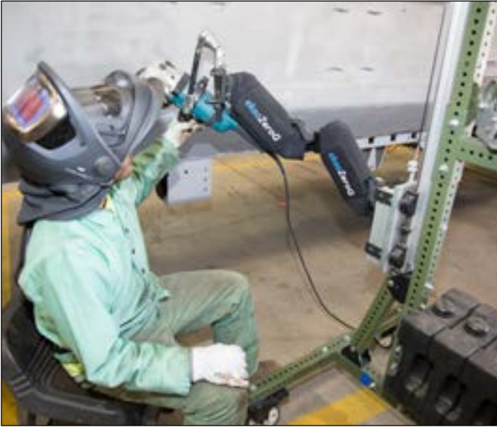
Niels Woods checks for a secure connection between the grinder he uses to smooth welds on an LAV and the zero gravity arm that counterbalances the weight of the tool, June 29, at Production Plant Barstow, Marine Depot Maintenance Command aboard the Yermo Annex of Marine Corps Logistics Base Barstow, Calif.
