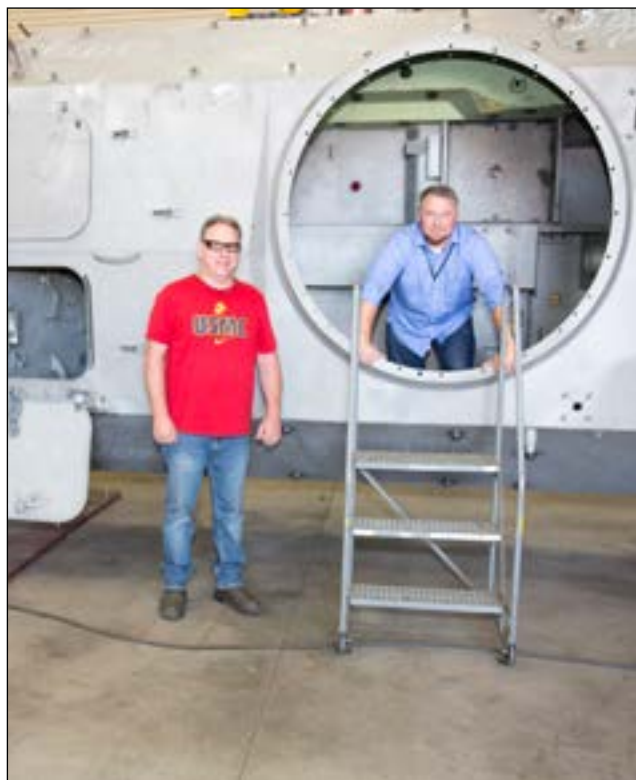
(Left) David Fritz, weld shop work leader, stands by as Ken Nowicki, weld shop supervisor, looks out of what is actually the top of a Light Armored Vehicle attached to the trunnion, June 29. The trunnion allows for positioning of the LAV to make welding joints much easier. The trunnion has been in use for four years at Production Plant Barstow, Marine Depot Maintenance Command aboard the Yermo Annex of Marine Corps Logistics Base Barstow, Calif.
