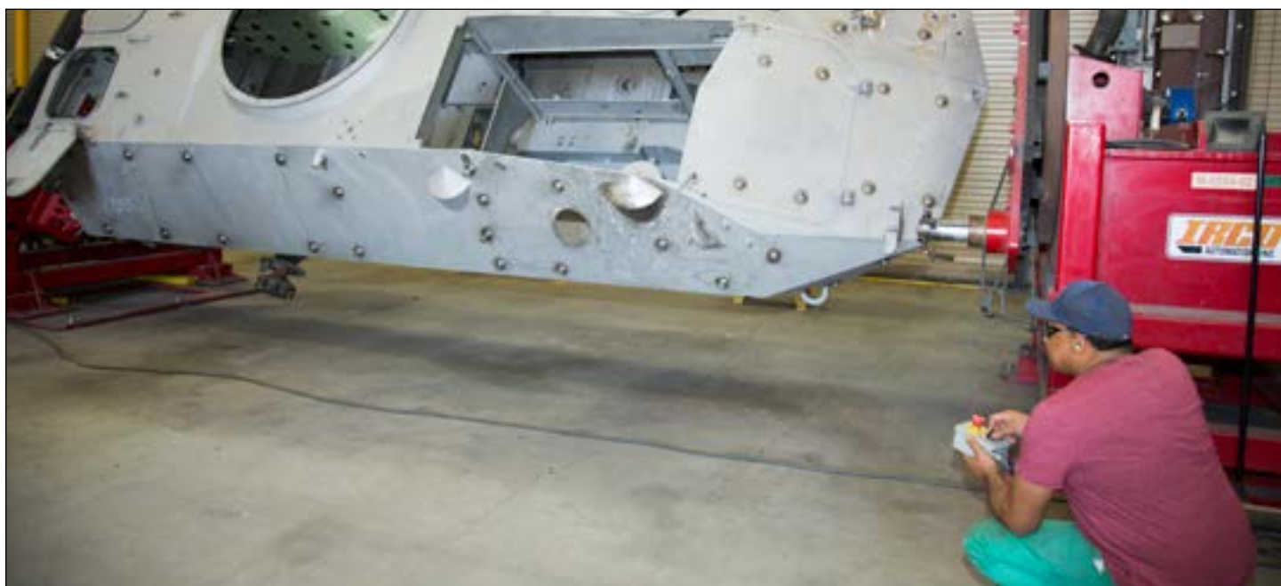
Eugene Dunford, welder, uses the controls to rotate the Light Armored Vehicle attached to the trunnion into a position to make it easier to make the numerous welds required at Production Plant Barstow, Marine Depot Maintenance Command, aboard the Yermo Annex of
