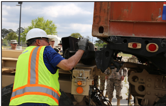
KBR personnel demonstrate how the new bracket mounts to the rear of a Conex Container making it work on the PLS trailer without a flat rack.
