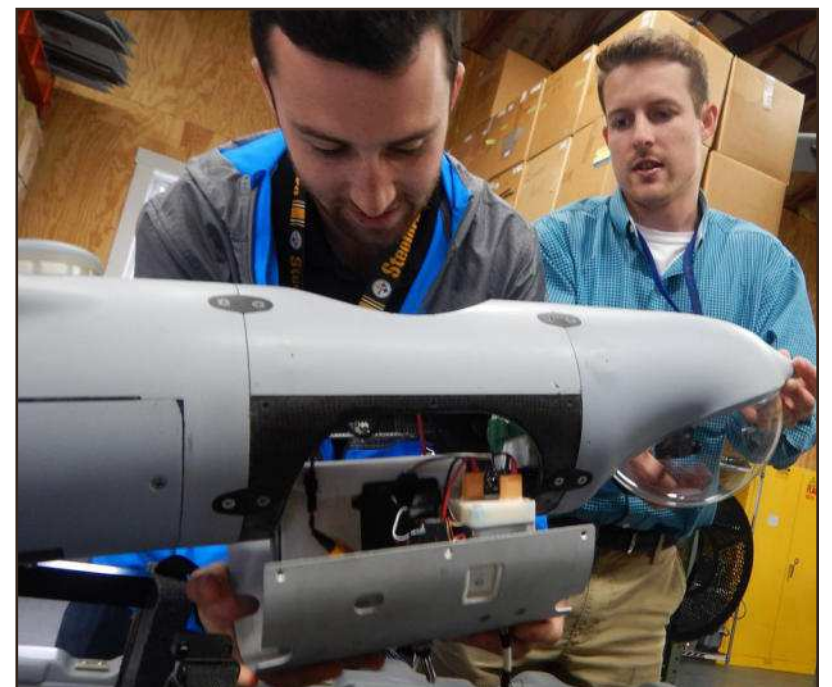
Navy scientist Jordan Lieberman, left, works with engineer Jonathan Crook to install the SCAPEGOAT payload onto a Boeing Insitu Scan Eagle unmanned aerial vehicle (UAV) prior to a system test flight. The SCAPEGOAT system — which includes modular interfaces to multiple chemical, biological, and radiological sensors and UAV platforms — was developed by junior scientists and engineers engaged in the Naval Surface Warfare Center Dahlgren Division-sponsored Sly Fox Program over a six-month period.
