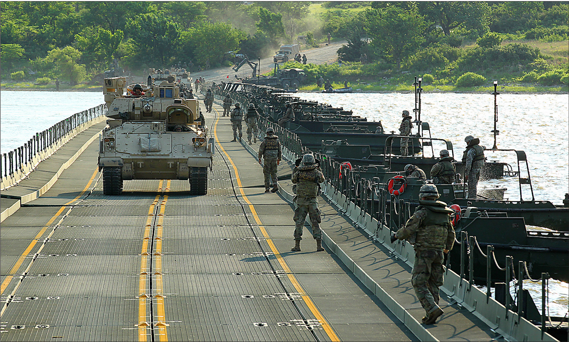
Chad L. Simon | 1st Inf. Div. Public Affairs A Bradley Fighting Vehicle crew works their way across the floating bridge on Milford Lake June 15. The 600-meter wet gap training was referred to as “Once in a lifetime” for some Soldiers.
