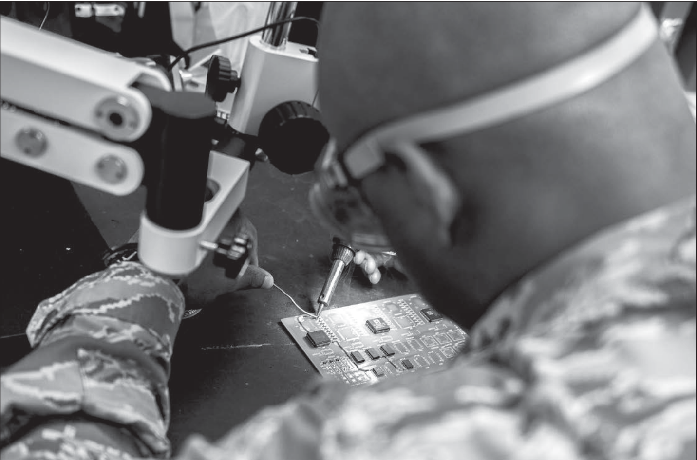
Senior Airman Darren Hopkins, a 354th Maintenance Squadron Air Force Repair Enhancement technician works on an aircraft circuit card May 29, 2018, at Eielson Air Force Base, Alaska. Hopkins is responsible for fixing and maintaining complex parts for many different aircraft. (Photo by Senior Airman Isaac Johnson, 354th Fighter Wing Public Affairs)
