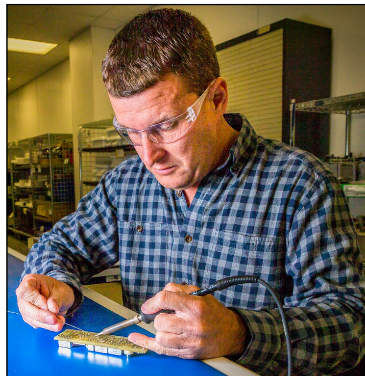
Forest Lester solders a component in the depot's Laser/Thermal Electronics Branch. Soldering and brazing are also forms of welding used each day at ANAD.
