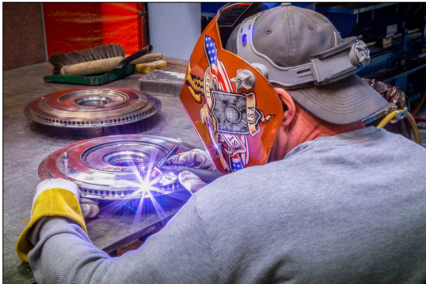
Gas tungsten arc welding is precision welding used on stainless steel, aluminum and titanium. Here, Shawn Garvey uses gas tungsten arc welding on parts for an AGT 1500 turbine engine.
