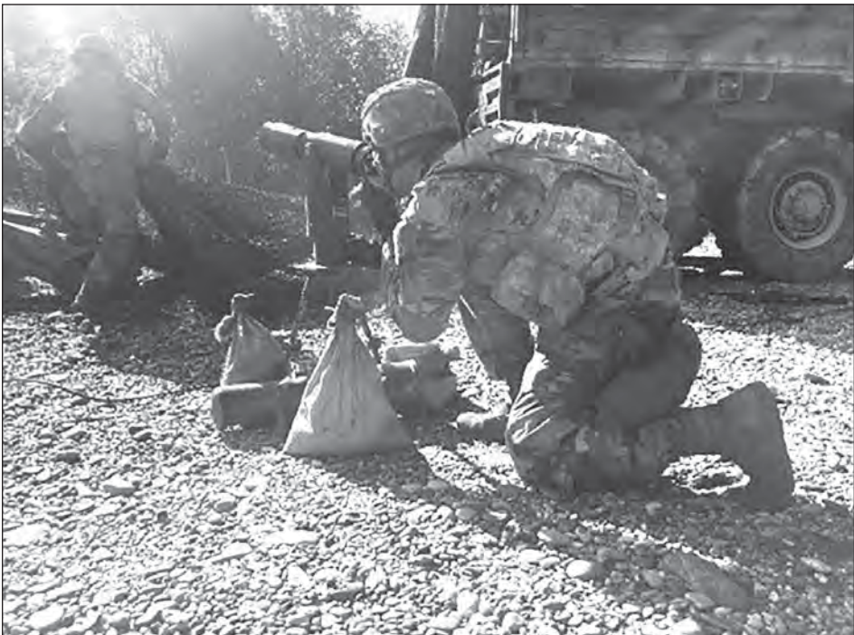
A Charlie Battery, 2nd Battalion 8th Field Artillery Regiment, 1st Stryker Brigade Combat Team Soldier sets up the collimator for the emplacement of a howitzer. (Photo courtesy, 1st Stryker Brigade, Combat Team, 25th Infantry Division)
