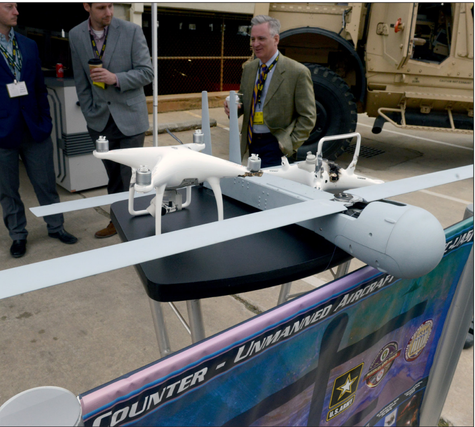
A Coyote Anti-Unmanned Aerial Systems Block 1B is on display at the Association of the U.S. Army's Global Force Symposium and Exposition, March 28, 2018 in Huntsville, Ala. The Coyote explodes on contact or near enemy UAS to take them out.
