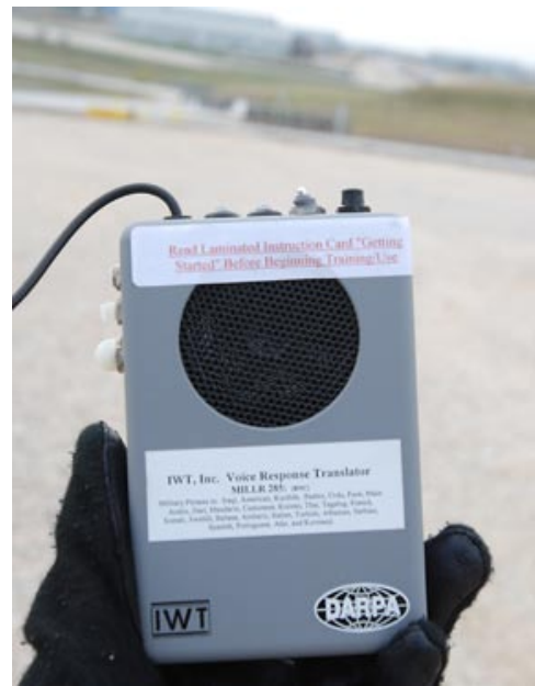
■ The voice response translator body weighs 11 ounces and is 3 inches wide and 4 3/4 inches long with a speaker on the front to project the phrases.
