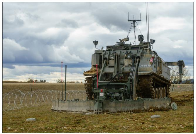
A U.K. Terrier armored digger clears a minefield and prepares to breach an obstacle during a Robotic Complex Breach Concept assessment and demonstration, at Grafenwoehr, Germany, April 5. The Terrier is a combat engineer vehicle capable of accomplishing combat and construction-engineering tasks while manned or remotely controlled.
