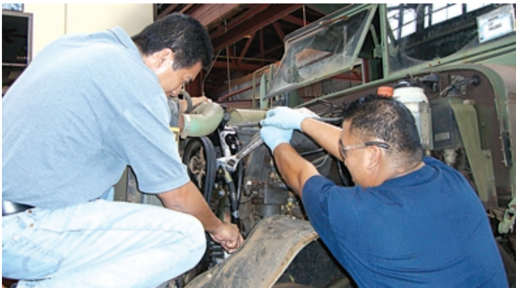
No matter how busy he is, Ricky Garcia always has time to help out a fellow colleague. Above, Garcia helps Glen Suniga replace the power steering on a military vehicle, the cargo truck M923A1.
