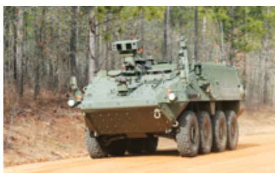
Crews drive the Stryker robotically through the Fort Gordon range, testing the unmanned vehicle making 68 turns on a 100-mile course.
