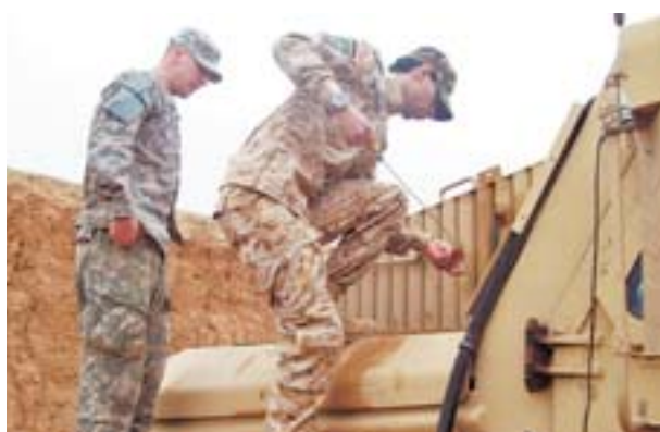
Spc. Derek Teunissen, 591st Engineer Company (Sapper), teaches an Iraqi army soldier how to operate the interrogation arm on a route clearance vehicle, to prepare him to conduct route clearance operations in the city of Mosul, Iraq.
