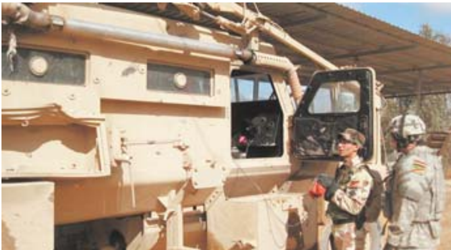
Spc. Derek Teunissen, 591st Engineer Company (Sapper), teaches an Iraqi army soldier how to operate the interrogation arm on a route clearance vehicle, to prepare him to conduct route clearance operations in the city of Mosul, Iraq.
