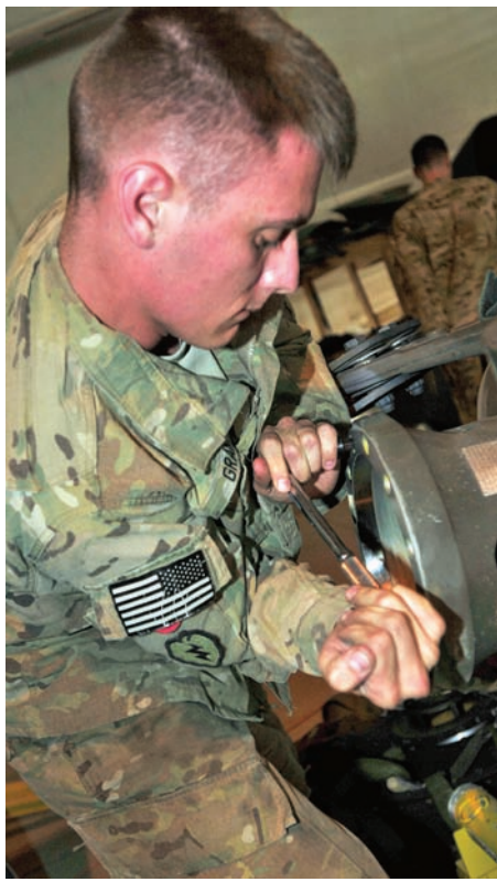
Spc. Christopher Grant, an aircraft powertrain repairer with Co. D, 2nd Bn., 25th Avn. Regt., 25th CAB, removes bolts from a main rotor hub for a UH-60 Black Hawk helicopter.
