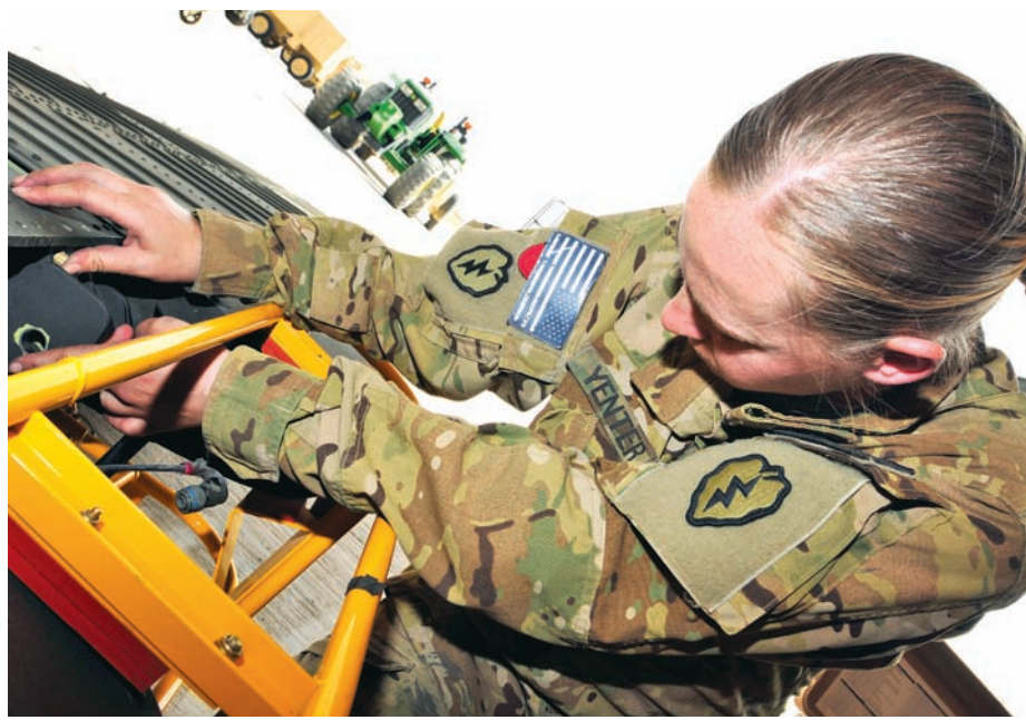
Spc. Melinda Yenter, a UH-60 Black Hawk crew chief with Co. D, 2nd Bn., 25th Avn. Regt., 25th CAB, installs stabilator hinge fitting on a horizontal stabilator for a UH-60 Black Hawk helicopter during a phase maintenance session in Afghanistan, recently.
