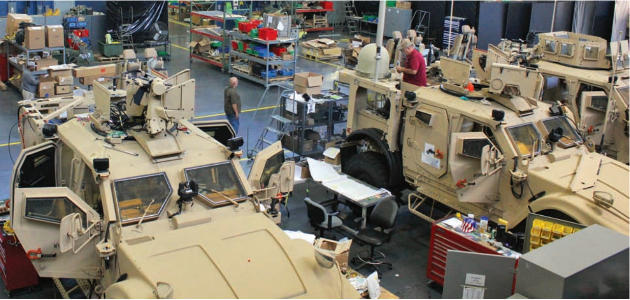
Pictured is the Prototype Integration Facility at the U.S. Army TARDEC, in Warren, Mich., where the first five “super configuration” MRAP prototype vehicles equipped with CS 13 assets are being built. The MRAP configurations include Soldier Network Extension, Point of Presence, Vehicular Wireless Package, MaxxPro and MRAP-Lite.
