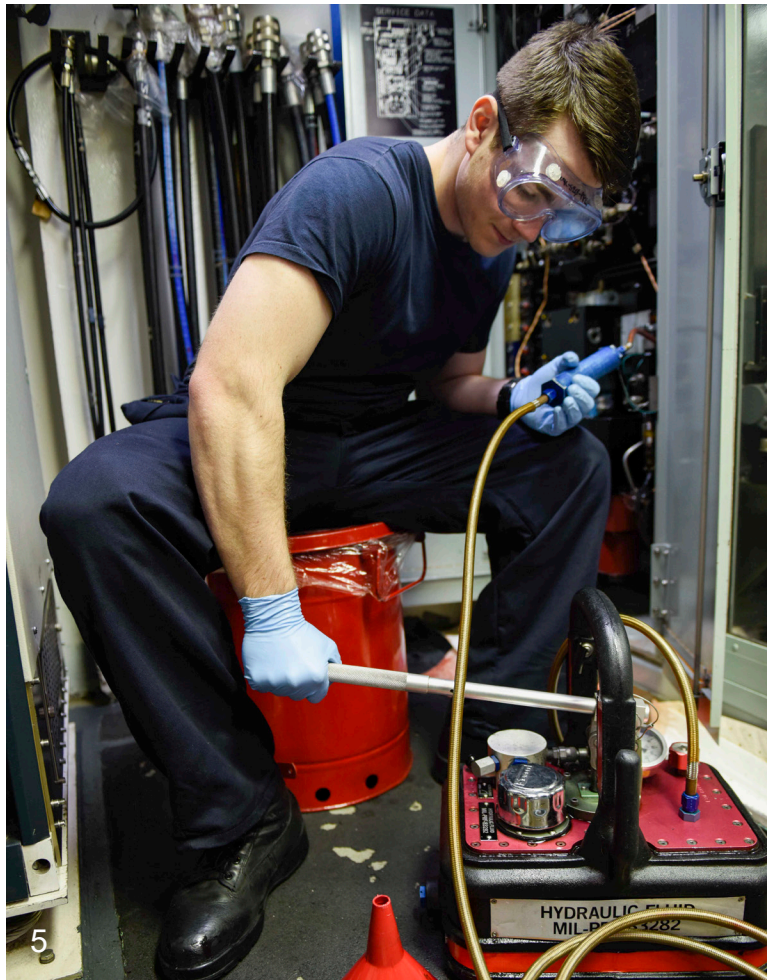
5. AMAN Joseph Somers fills a servo test stand with hydraulic fluid. Photo by MC3 Andrew Langholf.
