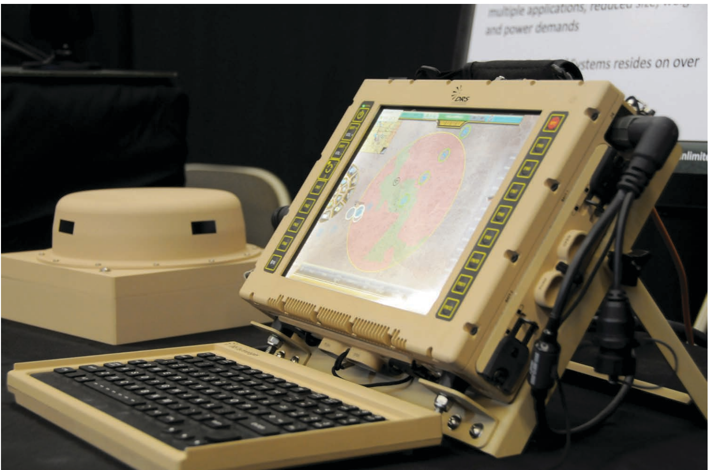
An Advanced Field Artillery Tactical Data System (AFATDS). (U.S. Army Acquisition Support Center)
