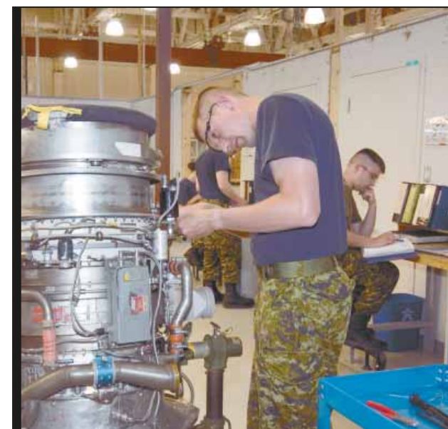
Cpl Steven Drinkwater (front), a candidate on the aviation systems technician course at CFSATE, finishes the lockwiring to complete the installation of an oil pressure transmitter on a J85CAN40 turbojet engine, while Pte Nathaniel Afonso (right) reviews the procedure.
