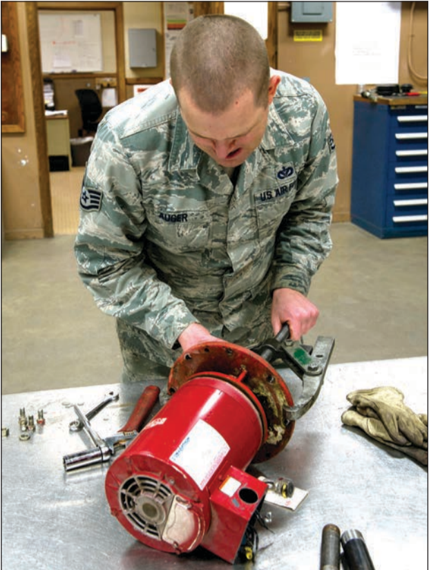
U.S. Air Force Staff Sgt. Matthew Auger, a 354th Civil Engineer Squadron heating, ventilation and air conditioning technician, repairs a leaking glycol pump Dec. 27, 2017, at Eielson Air Force Base, Alaska. The pump, which is essential to the building's heating system, required a new seal to stop the leak and return to normal function. (Photo by Airman 1st Class Eric M. Fisher, 354th Fighter Wing Public Affairs)
