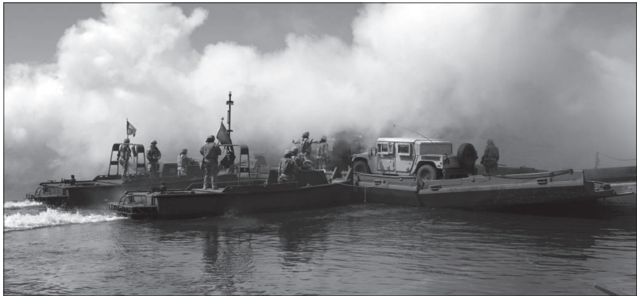
Army Reserve Soldiers from the 341st Engineer Company and 401st Engineer Company (Multi-Role Bridge Company) maneuver a six-bay float raft downstream on the Mississippi River at Fountain City, Wis., on May 7 as part of the 86th Training Division's Warrior Exercise 86-17-02.
