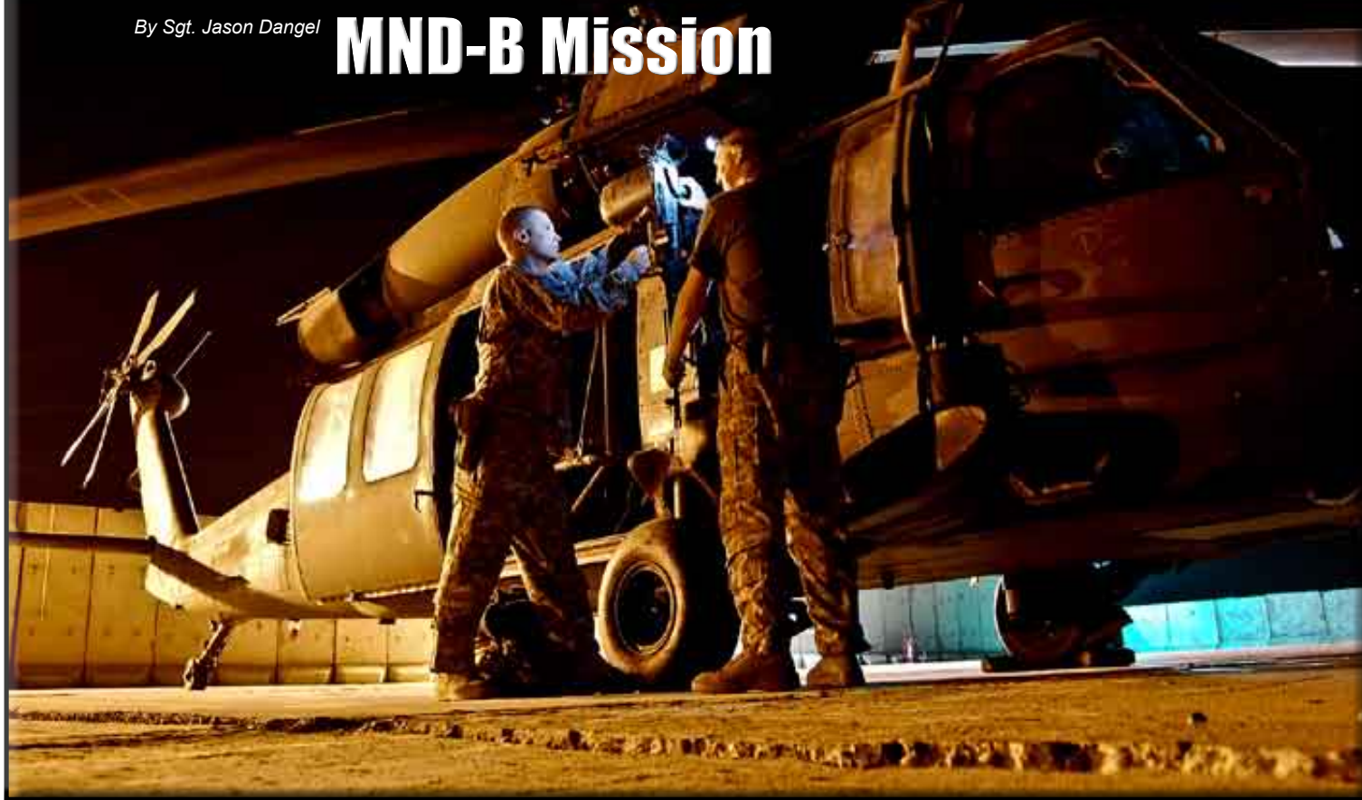
Sgt. David Brocato (left), crew chief, Co. C, 3rd Battalion, 4th Avn. Regt., CAB, 4th Inf. Div., MND-B, and counterpart Spc. Daniel Simonson (right), mount a M240B Machine Gun to the gunner's position of their Blackhawk helicopter before the start of a night mission on Camp Taji.
