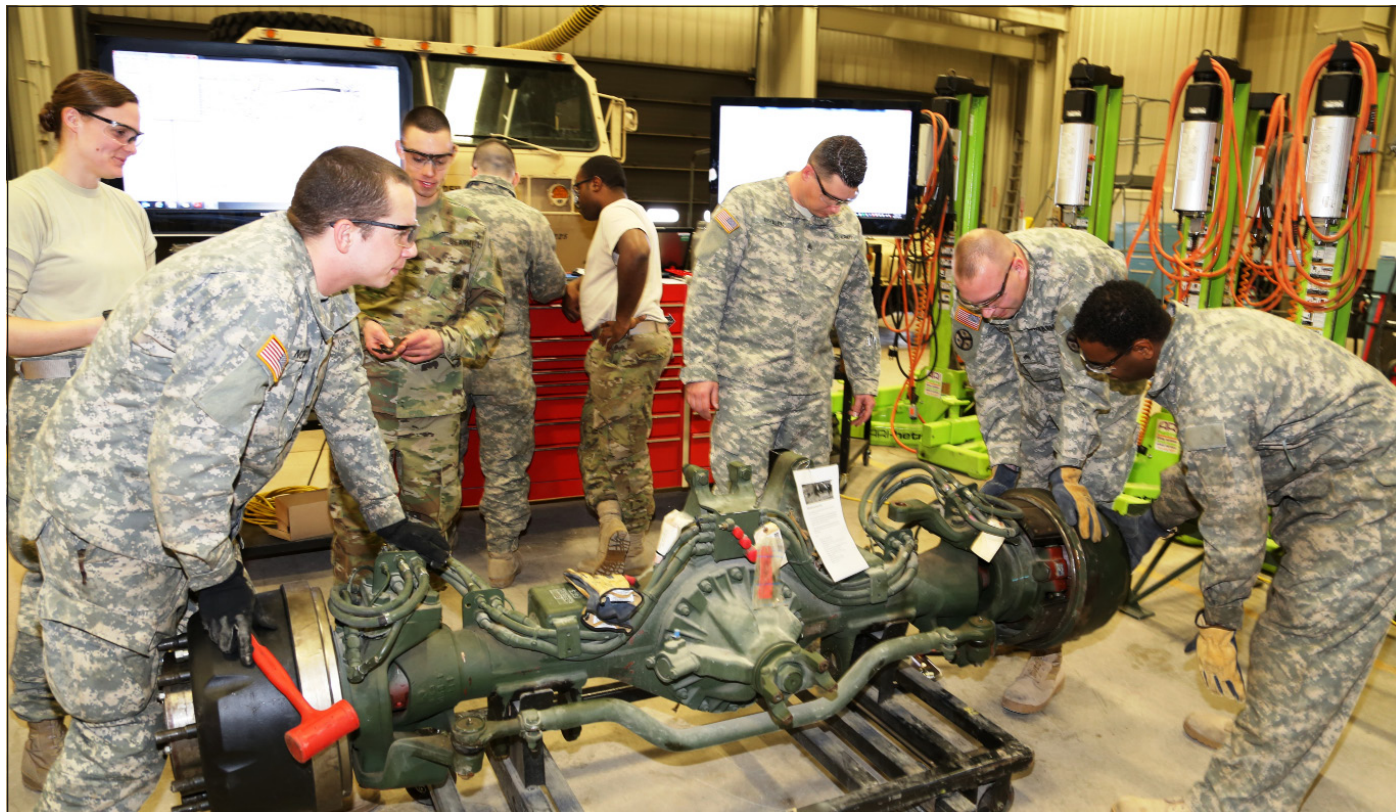
Students and instructors at Regional Training Site-Maintenance work on a project in the Wheeled Vehicle Mechanics Course on Feb. 10 at Fort McCoy. During the course, students learn to complete all basic concepts required to be certified as a wheeled-vehicle mechanic.
