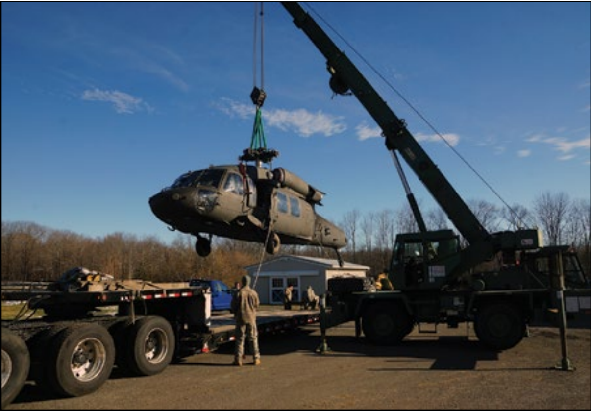
Members of the DART use a UTES 20-ton crane to load the dissasembled UH-60L Blackhawk Helicopter onto a heavy duty low boy in preparation for transport to the AASF, November 23. The aircraft was dissembled and moved following an emergency landing made by aviators of the Connecticut Army National Guard in South Salem, New York, November 20. (Photo courtesy of Command Sgt. Maj. Anthony V. Savino, 1-169th GSAB)
