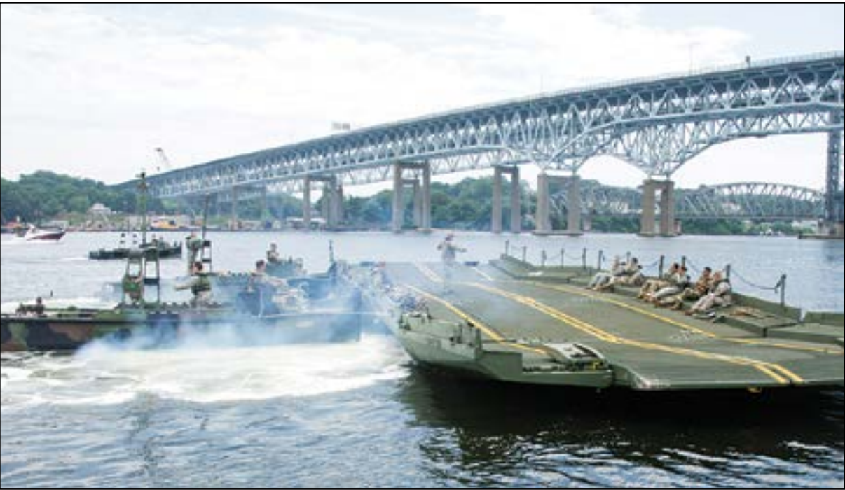
Members of the 250th Engineer Company (Multi-Role Bride Company) guide the Improved Ribbon Bridge with two Bridge Erection Boats across the Thames River during Sailfest in New London, Connecticut, July 8. The 250th participated in the 40th annual Sailfest event, a three-day festival that includes ship displays, carnival rides and a firework display on the waterfront of New London. (Photo by Staff Sgt. Richard Wrigley, JFHQ Public Affairs, Connecticut Army National Guard)
