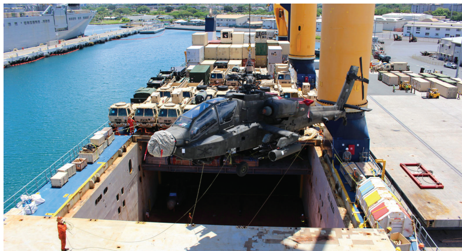
The forward ship's crane on the M/V Ocean Jazz lifts an Apache helicopter into the hold during port operations at Pearl Harbor on June 12.
