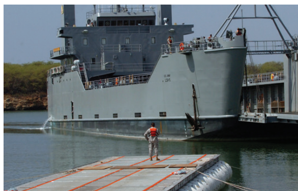
Logistics Support Vessel 5 floats in to connect its ramp, weighing about 30 tons, onto the Lightweight Modular Causeway System at Waipahu Peninsula. The LMCS is a prototype that can be used in many ways.
