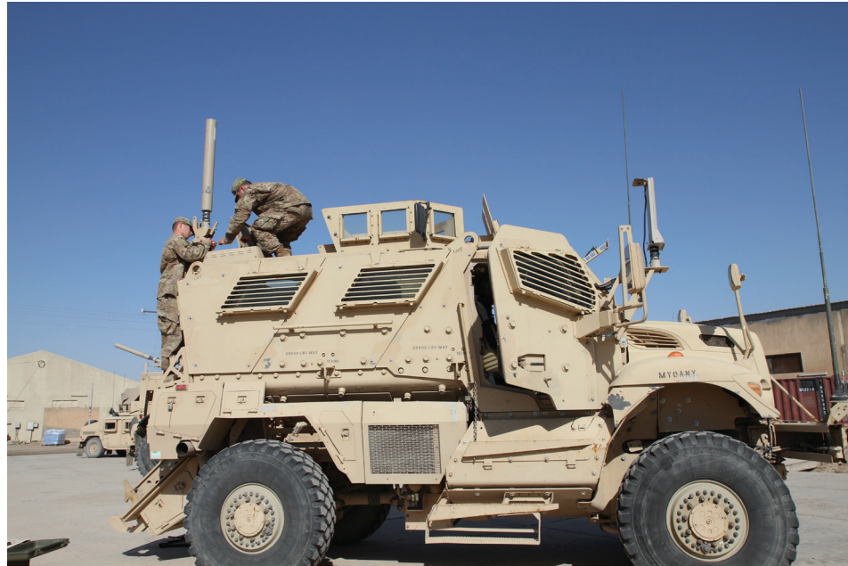
Sgt. Charles Smalley and Sgt. Alex Katz, both signal support systems noncommissioned officers with the 451st Expeditionary Sustainment Command, install a Blue Force Tracker system on a tactical vehicle for the 300th Sustainment Brigade Det. 2, Sept. 20, 2016 at an undisclosed location in Iraq. (Photo by Spc. Milagro Perez)
