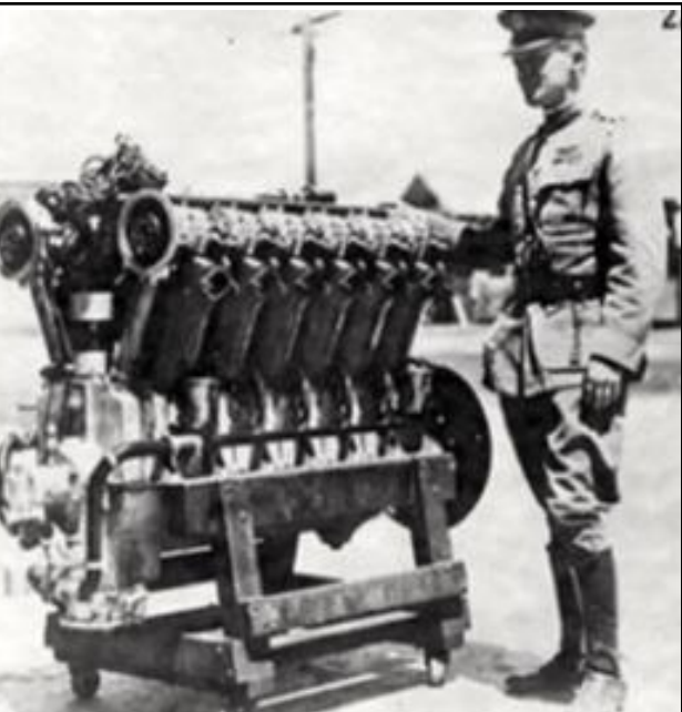
Just a month after America’s entry into World War I the government brought together leading engine builders to collaborate on the development of an advanced power plant, the result was the eight-cylinder Liberty engine; the first production engine is shown here next to future GEN “Hap” Arnold. (source: USAF)
