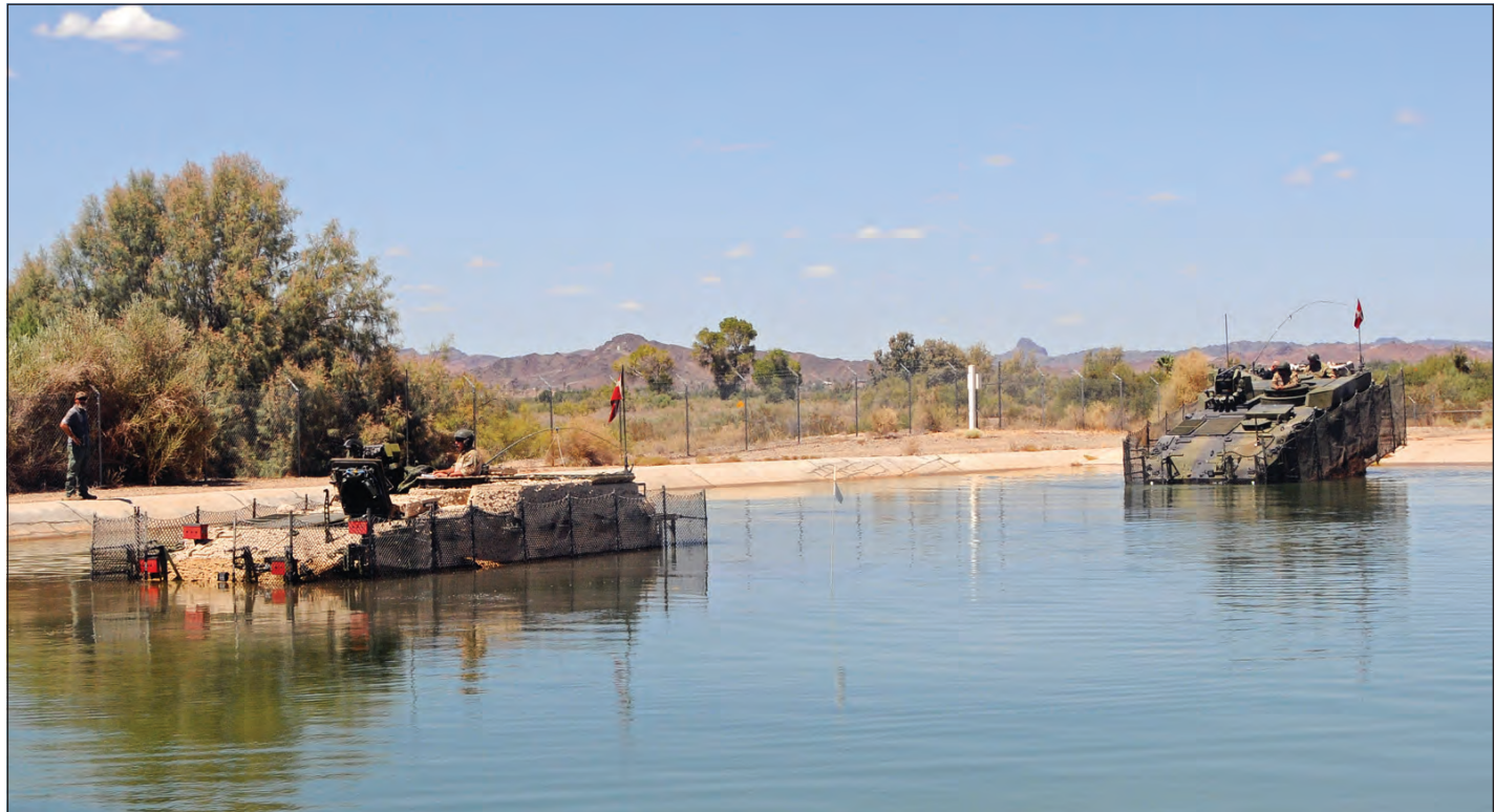
Two Piranha 5 infantry fighting vehicles undergoing a test at YPG conducted by the Danish Defense Acquisition and Logistic Organization traverse a fording basin as part of a month-long test in August. The test at put the base infantry variant of the Piranha through its paces across punishing desert terrain. (Photo by Mark Schauer)
