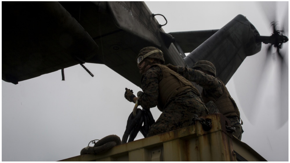
Pfc. Tyler J. Nye (left) and Cpl. Tyler D. Reed (right), both landing support specialist, prepare to attach a container to a CH-53E Super Stallion during external lifts training at Draughon Range near Misawa Air Base, Japan, August 21, 2017, in support of exercise Northern Viper 17. Nye, a Lincoln, Nebraska native, and Reed, a Waukesha, Wisconsin native, are assigned to Combat Logistics Battalion 4, Combat Logistics Regiment 3, 3rd Marine Logistic Group.
