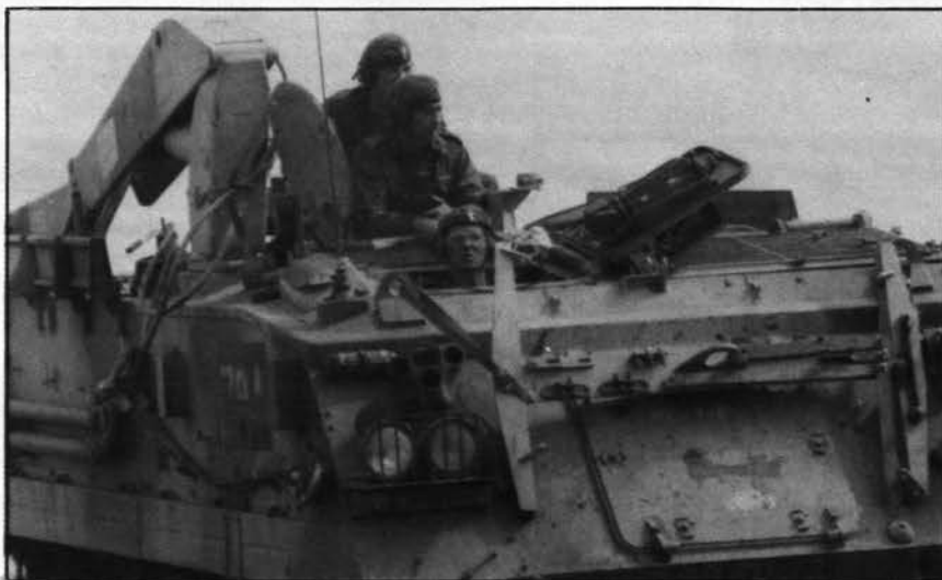
A Royal Electrical & Mechanical Engineer (REME) FV434 mounting a HIAB crane waits in readiness to recover bogged or damaged vehicles at Suffield during the British Army Training exercises there.
