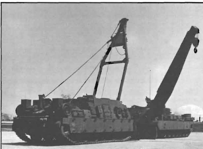
Aberdeen Proving Ground is testing two candidates for the Army's new recovery vehicle. At left is the modified M88A1E1, built by BMY, manufacturer of the current M88 series. At right is the General Dynamics entry, based on the M1 tank chassis.
