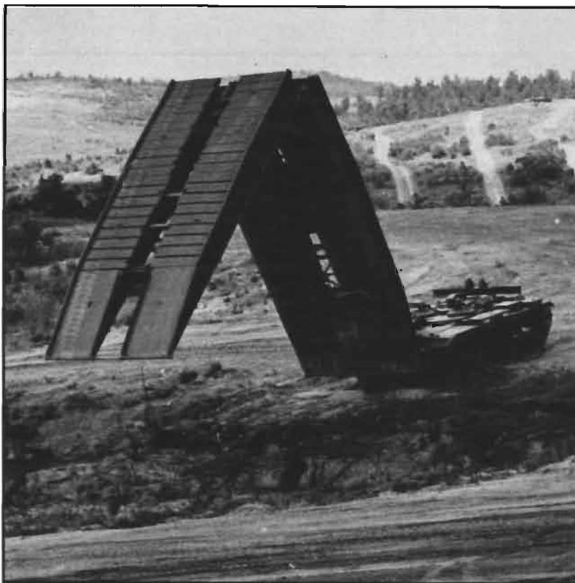
Current Armored Vehicle Launched Bridge, mounted on M60 chassis, is too slow to keep up with M1 units and presents weight restrictions.
