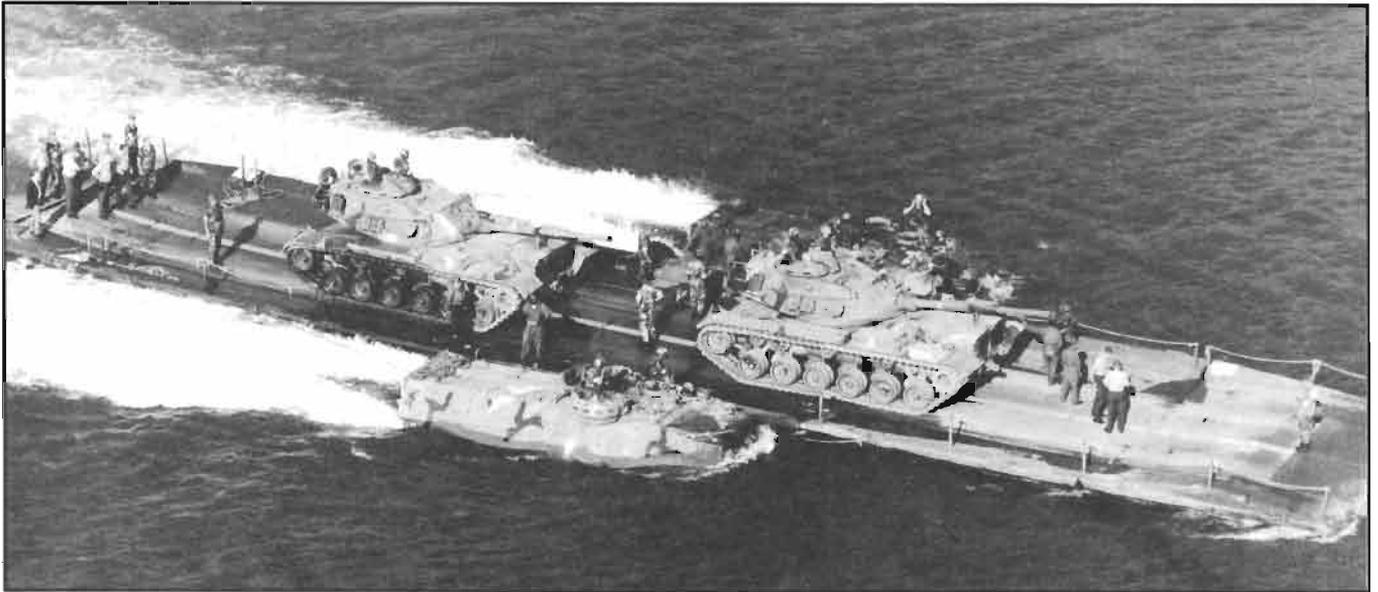
Interior and ramp sections of Ribbon Bridge can be joined to provide rafts for heavy combat vehicles.
