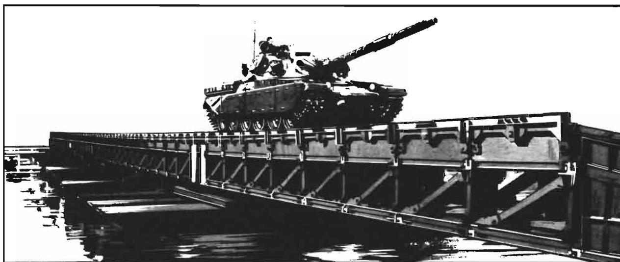
The Medium Girder Bridge can be deployed to span a wide body of water.
