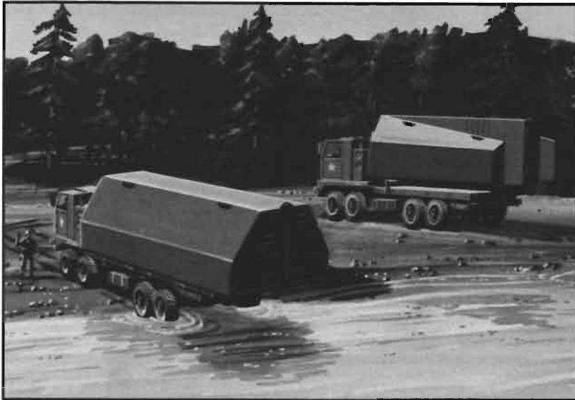
The Improved Ribbon Bridge, seen in an artist's rendering, above, as it prepares to deploy from its transporter-launcher.
