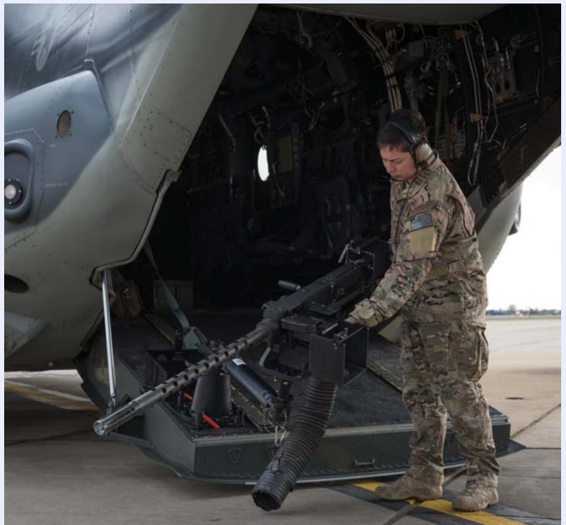
U.S. Air Force Staff Sgt. Justin O'Brien, 7th Special Operations Squadron special mission aviator, performs preflight checks on a CV-22 Osprey's ramp-mounted weapon system, a .50-caliber GAU-21 heavy machine gun Mar. 7, on RAF Mildenhall, England. When assigned to the tail position of the aircraft, SMAs are responsible for operating the RMW, weight and balance, clearing the landing zone and alternate insertions and extraction methods, among other duties. Photo by U.S. Air Force Capt Chris Sullivan.
