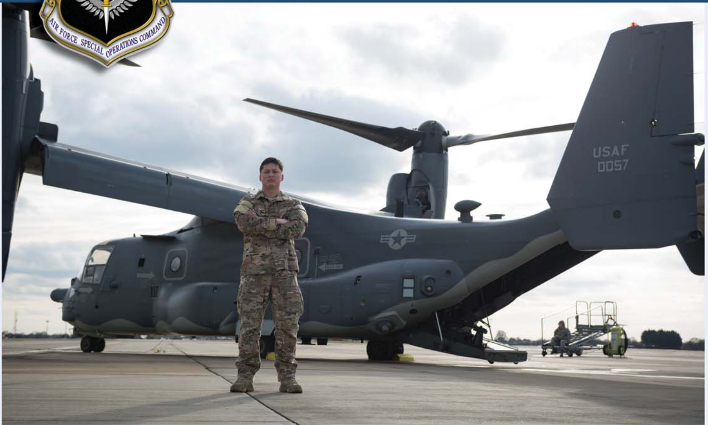
U.S. Air Force Staff Sgt. Justin O'Brien, 7th Special Operations Squadron special mission aviator, stands in front of a CV-22 Osprey Mar. 7, on RAF Mildenhall, England. The CV-22 is a tiltrotor aircraft that combines the vertical takeoff, hover and vertical landing qualities of a helicopter with the long-range, fuel efficiency and speed characteristics of a turboprop aircraft. Photo by U.S. Air Force Capt Chris Sullivan.
