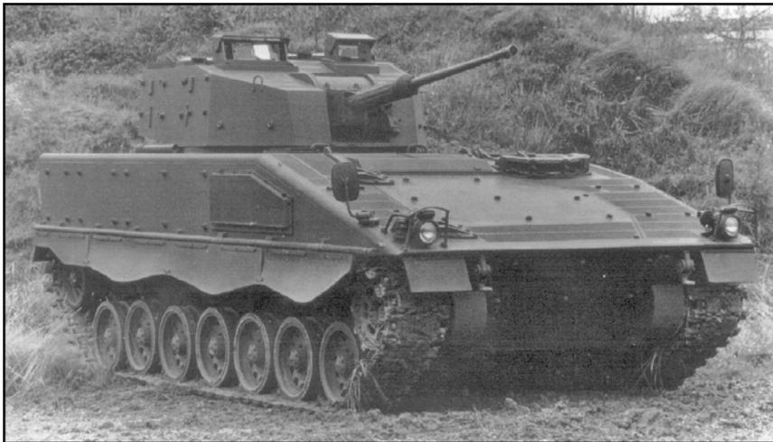
The Ascod tracked IFV, above, is a joint Austrian-Spanish collaboration. Its turret mounts a 30mm Mauser dual-feed automatic cannon.
