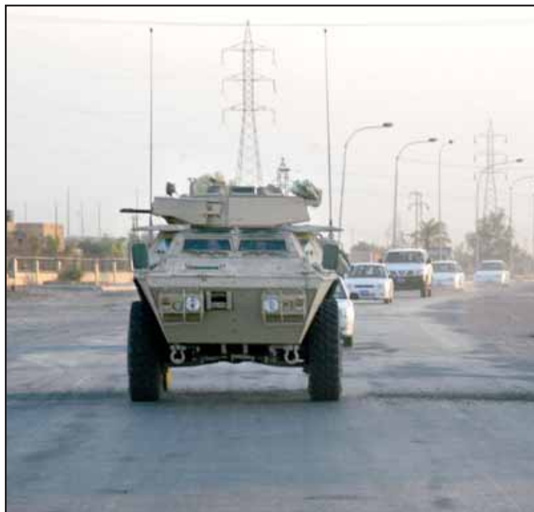
"The increased protection of the M1117, combined with a fully enclosed turret and 360-degree observation from inside the vehicle, greatly increases the crew's ability to rapidly and effectively engage targets. The Guardian is equipped with the dependable firepower provided by the Cadillac Gage™ up-gunned weapons station, consisting of an MK-19 40mm grenade launcher and .50-caliber machine gun."
