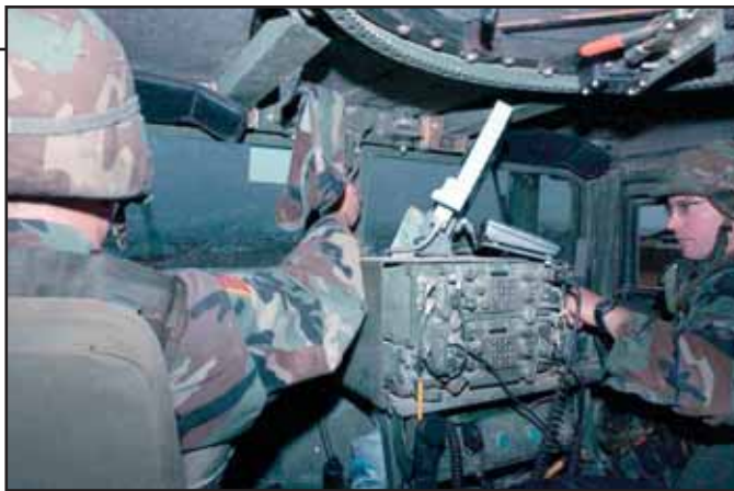
"When FBCB2 was fielded in the mid-1990s, it was heralded for its capabilities. FBCB2 combined global positioning satellite (GPS) capabilities, computers, and tactical radio-based networks, allowing soldiers to communicate horizontally (between platforms) and vertically (to tactical operations centers) to automatically share their position reports on a common operational picture."
