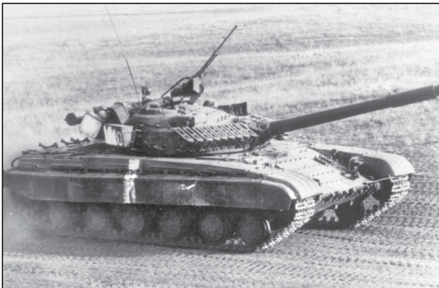
"In 1966, the Russians developed composite armor technology, known as combination K, in its T-64 main battle tank. Early T-64 armor used a layering of steel reinforced with glass fibers embedded in a plastic material "sandwiched" between the steel plates. Later, T-64s substituted a boron carbide ceramic material that was much more resistant to HEAT penetration. The theory of composite armor is it is stronger and lighter than steel and it dissipates the HEAT jet and/or breaks up a hardened steel armor piercing round (kinetic energy (KE)), preventing penetration into the inner armor plate."
