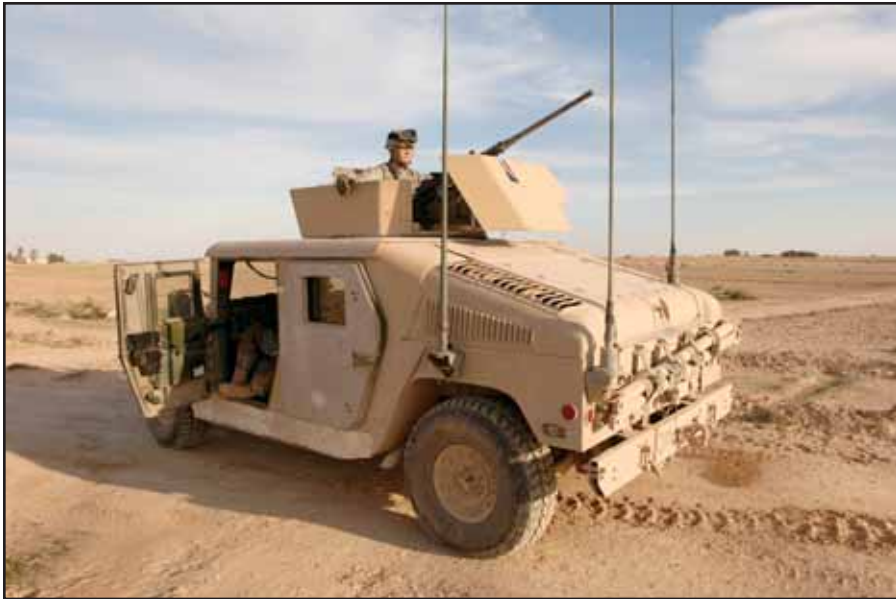
"The M1114 was designed primarily for an environment where it would be expected to operate on roads due to a far-reaching land mine threat; therefore, the vehicle is inadequate as an off-road vehicle. It loses its ability to move rapidly off-road and must travel extremely slowly on restrictive terrain."
